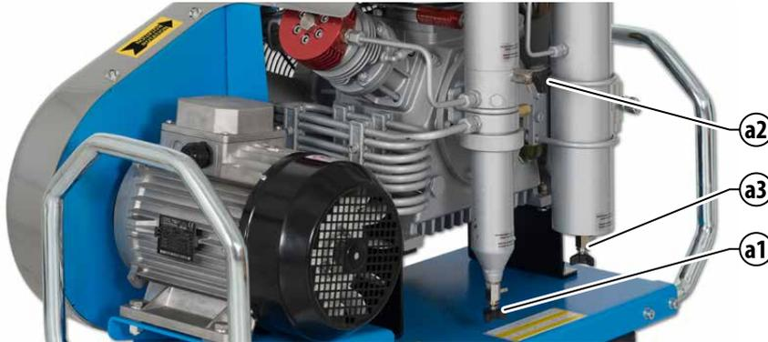
For compressors with automatic condensate discharge the condensate discharge occurs automatically every 7 minutes. The yellow TEST PURGE pushbutton (b) must be pressed every day to make sure that the discharge valve is working properly.
